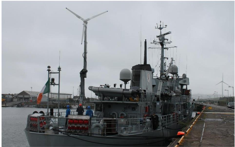
DARE Tech offsetting diesel energy in port. Image courtesy of DARE Technology
